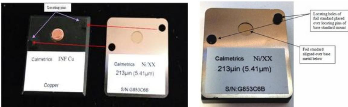
Foil standard placed over base standard mount with foil aligned over base metal
