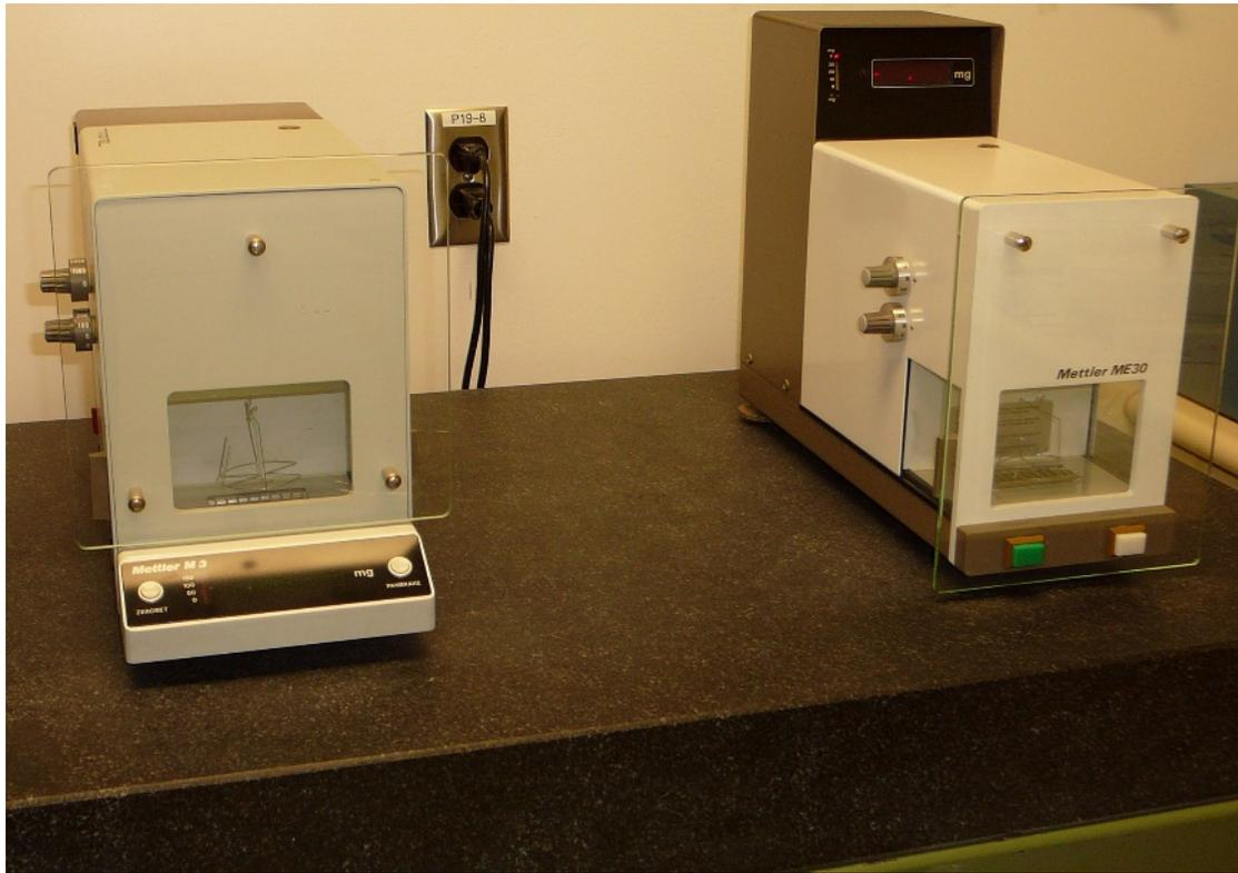
**Fig. 1: Micromatter Precision Balances**
