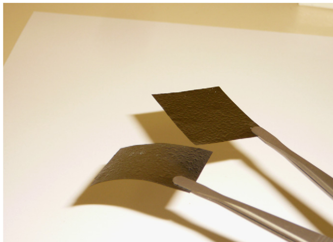
Fig. 1. Comparison of DLC–B–DLC foil (left, flexible) and DLC–Si–DLC foil (right) of equal thickness.
